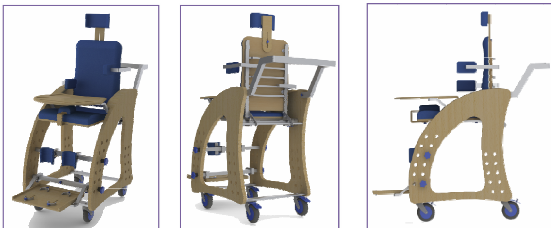
Figure 3.3. Modular wheelchair in position for seating
