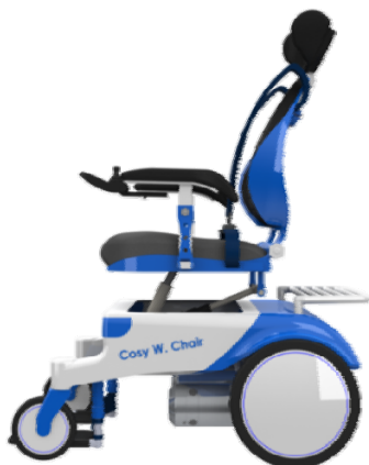
Fig.3.3.5 Elevated position of the seat
